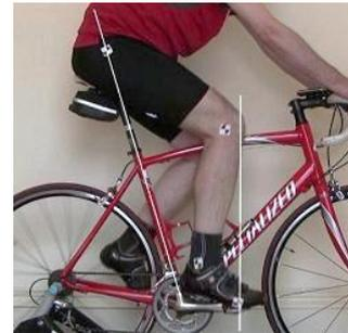
It can work very well though because it is a good predictor of the hip position relative to the seat tube axis. If the hip joint is along this axis, the rider will tend to be well balanced without too much weight on their hands and as the bike designer intended.
